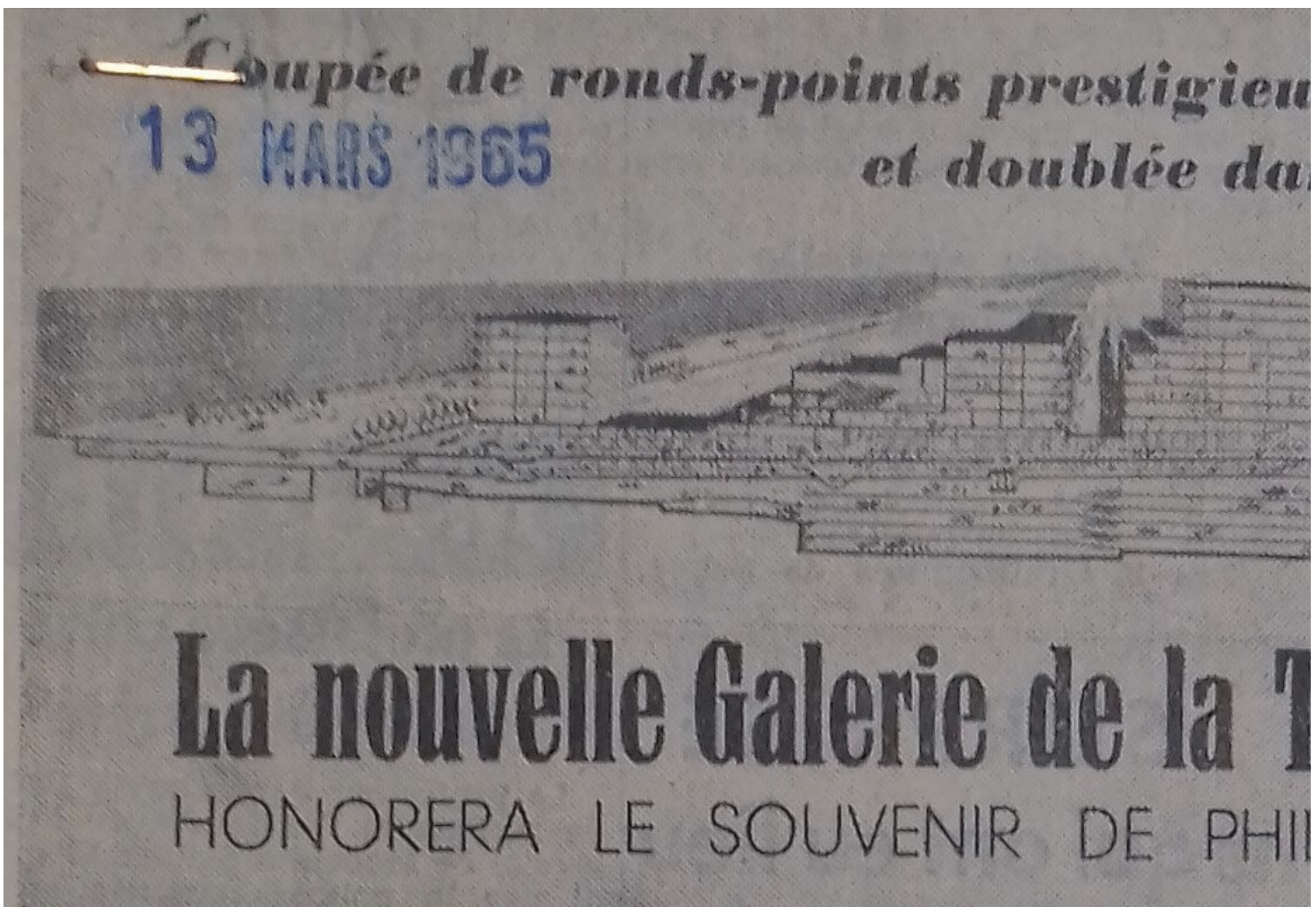
Figure 4 Cross-section of the Toison d'Or Gallery illustrating the multiplication of ground levels and the fine connection of rapid mobility infrastructures with the architectural complex (metro access, parking, motorway tunnel). Source: André Hustin, "The new Toison d'Or Gallery will honour the memory of Philippe le Bon. Punctuated by prestigious roundabouts and doubled in height", March 13, 1965, p.1. © KBR.
