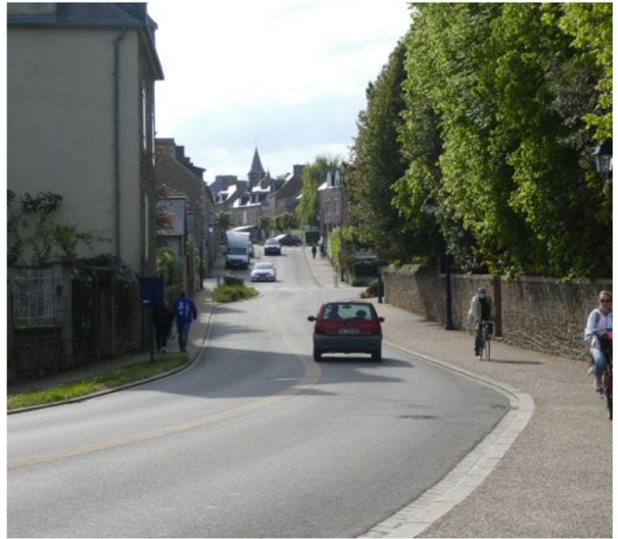
Figure 5: Example of a departmental road that has been adapted to promote and ensure the safety of active mobility: wide cycle way on the side, lit at night, separated from the road and running continuously through villages (Pierre Helwig).
