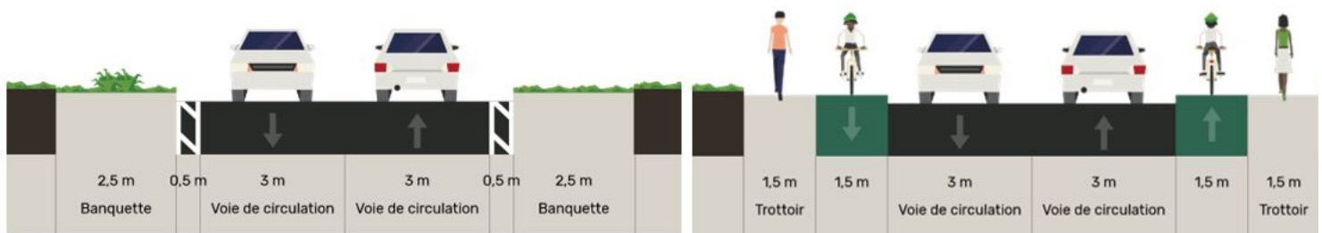
Figure 4: Adapting the sides of departmental roads should accommodate soft modes, including outside of towns and villages (Pierre Helwig with Streetmix)
